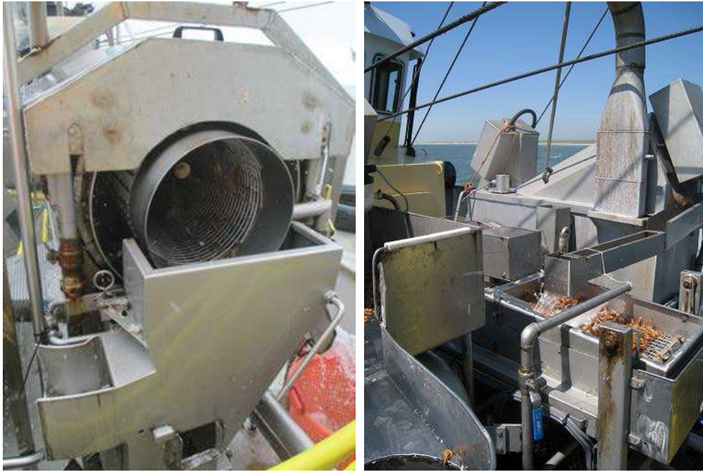
Figure 43 Sieving devices on board of shrimp vessels: coaxial sieving drums (left), trembling sieve (right) (Source: Steenbergen et al, 2015).
